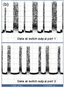
Fig. 19. A fast switching example of asynchronous data. (a) The initial data stream and the header in front of the payload. (b) The switched data as they appear at two output ports of the switch.
