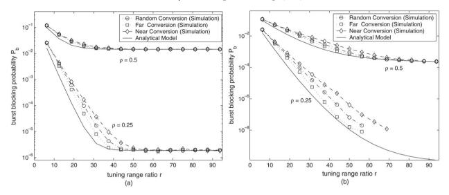
Fig. 6. Blocking probabilities for K=32 with respect to the tuning range ratio parameter r for two different values of  $\rho=0.25$  and  $\rho=0.5$  when (a) W=15 and (b) W=25.
