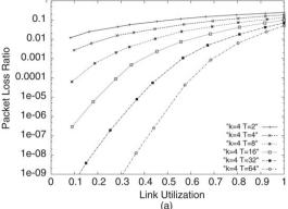
Fig. 17. Switch loss ratio for (a) k=2 and (b) k=4 versus link utilization for  $T \in [2...64]$ . Burst arrivals and idle periods follow a truncated Pareto distribution with a tail index of 1.7 and 1.2 respectively.
