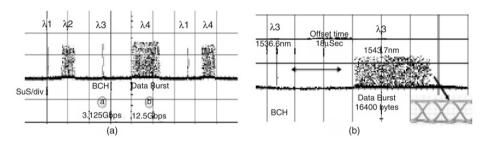
Fig. 21. Experimental result of the OBS transmitter.
