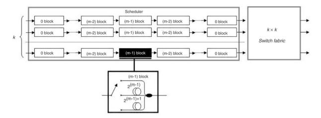
Fig. 16. The Scheduling switch; a feed-forward delay based switch architecture. The Scheduler comprises k branches, each with  $2 \log_2 T - 1$  delay blocks. The ith delay block consists of one three-state switch and three delay lines of length 0,  $2^i$  and  $2^{i+1}$  packet slots.
