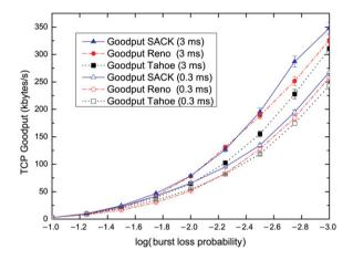
Fig. 11. TCP goodput vs. burst loss probability.
