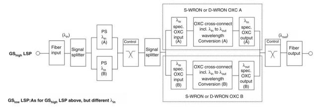
Fig. 15. Availability block diagrams for BE traffic and GS traffic.
