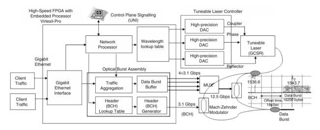
Fig. 20. Architecture of a wavelength agile edge optical burst switching interface.
