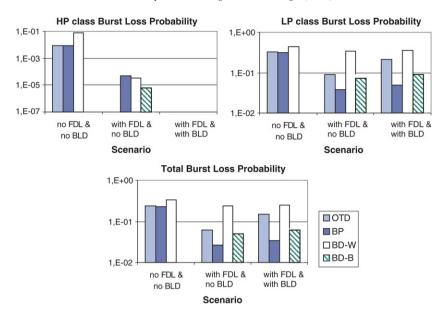
Fig. 12. Comparison of selected QoS mechanisms with and without FDL and BDL techniques.
