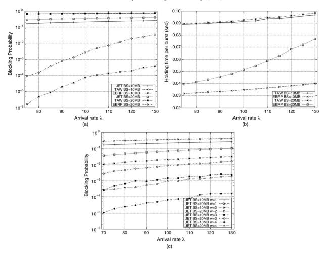
Fig. 2. (a) Blocking probability and (b) holding time of burst at network edge for JET, TAW, EBRP in a single channel network. (c) JET blocking performance for different numbers of wavelengths per fiber, assuming full wavelength conversion switches.
